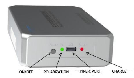
The CS100 is internally powered by a lithium battery, which can be placed in a glove box or used outdoors. The lithium battery can be charged in advance, and the Type-C interface is used for charging and communication. The circuit adopts a floating-ground design, and the electrochemical parameters of the grounding system can be measured without an isolation transformer.
