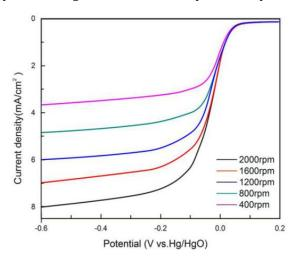
LSV: mesoporous carbon material in 0.1M KOH
