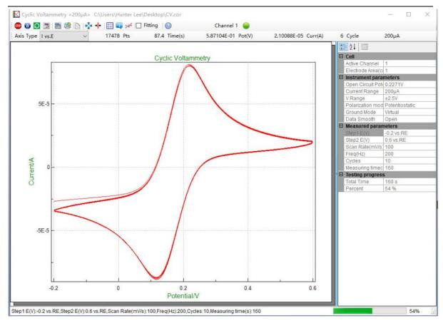
CS studio also provides powerful non-linear fitting on Butler-Volmer equation of polarization curve. It can calculate Tafel slope, corrosion current density, limitation current, polarization resistance, corrosion rate. It can also calculate the power spectrum density, noise resistance and noise spectrum resistance based on the electrochemical noise measurements.
