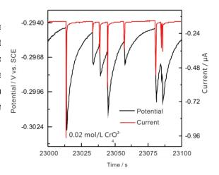
Electrochemical noise of low-carbon steel in 0.05mol/L Cl<sup>-</sup>+0.1mol/L NaHCO<sub>3</sub>
