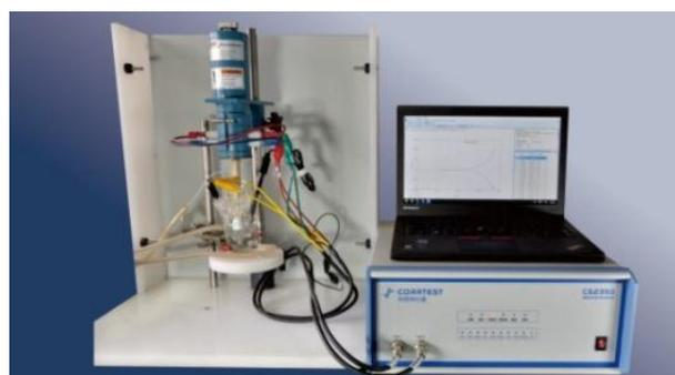
intermediate products on the disk electrode. RRDE test becomes the typical method for ORR study. CS2150 can be connected to a RRDE equipment from Pine or ALS. We can supply RRDE-3A setup (100 to 8,000 rpm rotating rate, ALS, Japan) with our bipotentiostat.
