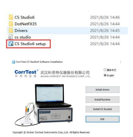
3. Firstly, install the drivers. After finishing it, go to the computer management → device manager → Ports (COM & LPT). There, it will appear "Silicon Labs CP210x USB to UART Bridge(COM x)". As is shown below, the X is 3.
