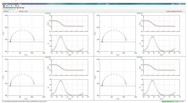
You can also choose different techniques in each channel. Set the parameters for each experiment one by one, and run each experiment independently. As is shown in right picture, EIS, Galvanostatic charge & discharge, Cyclic Voltammetry, and polarization curve test are tested.
