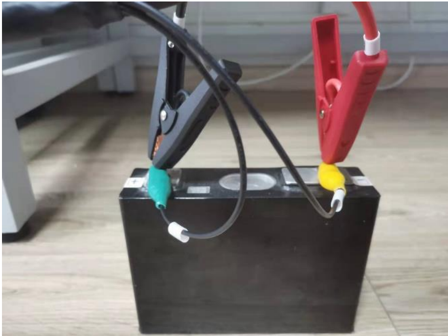
Fig. 2: Connection of CS2020B with battery core anode and cathode
