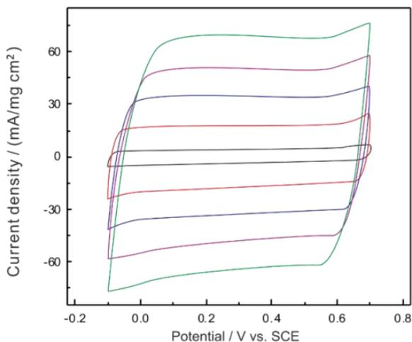
CV of PPy supercapacitor in 0.5 mol/L H<sub>2</sub>SO<sub>4</sub>
