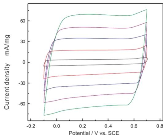
CV curve of PPy supercapacitor in 0.5 mol/L
