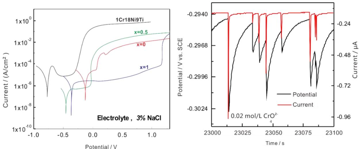
Polarization curves of Ti-alloy& stainless steel in 3%NaCl solution(left)
