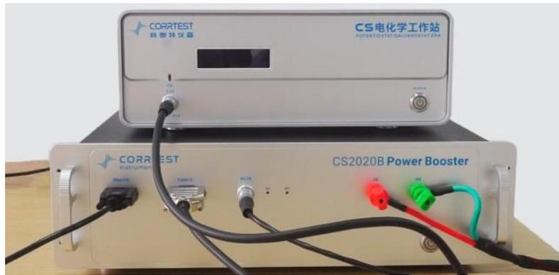
**DB9 cable:** one end inserts into Misc. I/O on back panel of potentiostat, the other end inserts into Misc. I/O on front panel of CS2020B.
