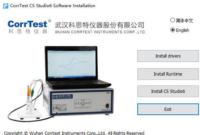
3. Firstly, install the drivers. After finishing it, go to the computer management → device manager → Ports (COM & LPT). There, it will appear “STM... virtual COM Port(COM x)”. As is shown below.
